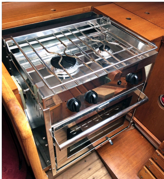
The Force 10 Euro Compact stove, as installed aboard OWL. The lever under the oven door actuates the gimballing feature. The door itself locks securely, and retracts as it opens thanks to a clever hinging mechanism. All burners feature electronic ignition.
